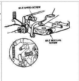
It is important to follow all linkage and lever installation instructions. The number one and two reasons for tuning errors are improper linkage installations and over tightened linkage nut, causing a binding in linkage assembly.
