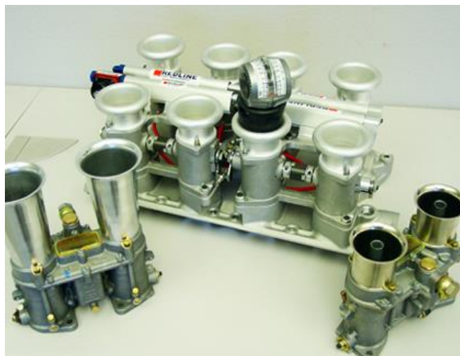
STE BK used with V8 injection And Weber 48-IDA's
